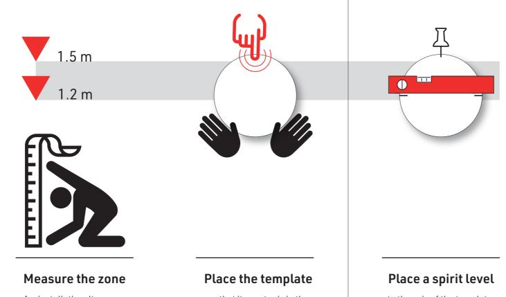
for installation. Its upper boundary will be at a height of 1.5 m and the lower boundary at a height of 1.2 m. Perfect
