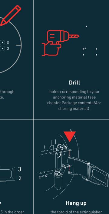
ne toroid of the extinguish to the pins of the holder.
